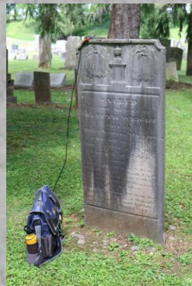
Figure 5: GIS data collection in the field using an ArrowLite GLONASS GPS Receiver
